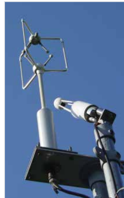
Eddy covariance system, which measures crop evapotranspiration data to help evaluate soil water content.
