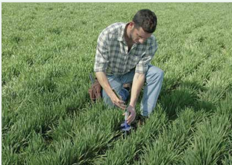
Farmer deploying wireless soil water content sensor in field. Credit: PrecisionAg
