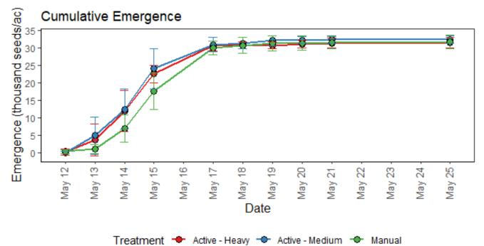
**Figure 1.** Cumulative emergence by date for manual downforce, active downforce at medium pressure, and active downforce at heavy pressure.
