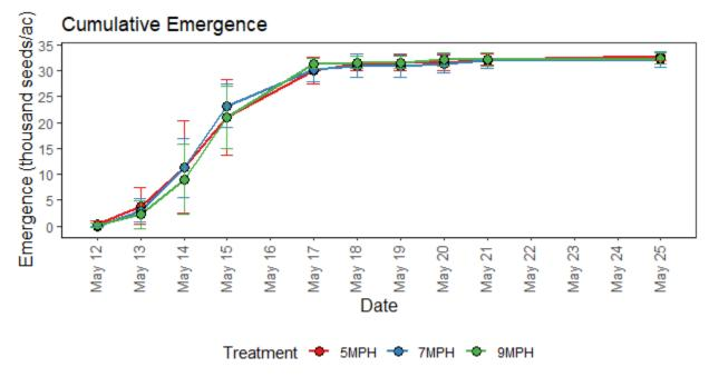
Figure 1. Cumulative emergence by date for 5 mph, 7 mph, and 9 mph planting speeds.
