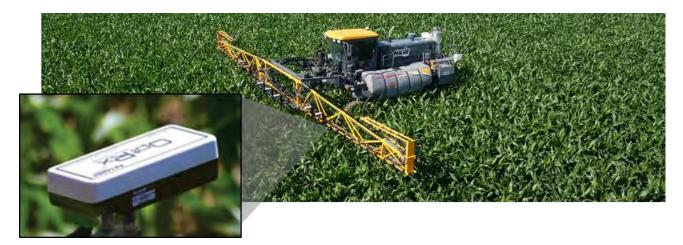
Figure 1: Active crop canopy sensor (left) positioned over the corn canopy and high-clearance applicator (right) equipped with OptRx<sup>®</sup> crop canopy sensors, GPS, and drop nozzles.
