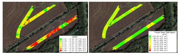
**Figure 1.** NDRE values from Ag Leader<sup>®</sup> OptRx<sup>®</sup> sensors (left) and variable-rate nitrogen directed by sensors (right) applied on April 21, 2021. 108 | 2021 Nebraska On-Farm Research Network
